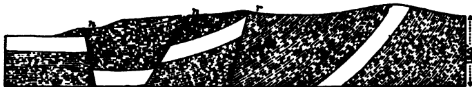
Fig. 14. Faults in strata, near Forty Mile, Yukon river, Alaska; nn.—normal faults; r.—reversed fault. After J. E. Spurr.*
